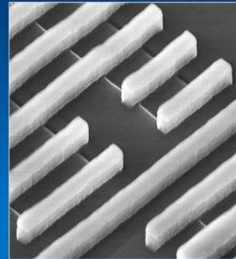
22 nm Tri-Gate Transistors
