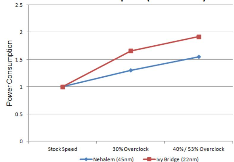
Higher temperatures result from a smaller die size as well as a larger transistor density. Also the increased transistor density results in a larger overall resistance, which means more power is required to overclock the chip.
